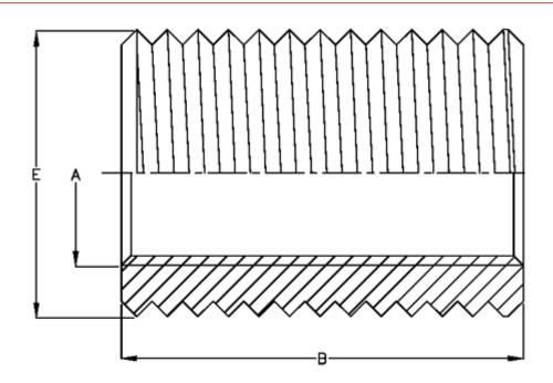
Female thread A = M6Length B= 12Male thread E= M8Type= 97x 000 060.120
